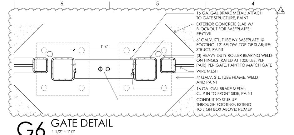
SKUK I WE EUWREEX BRAKE METAL INFILL RE: G6/A1.04 6" STL STRUCTURE 4" STL GATE FRAME 4" GALV WIRE FABRIC HEAVY DUTY HINGED HASP (STANLEY 517600 OR ACCEPTED SUBSTITUTE) STAINLESS STEEL ROUND GRIP PULL HANDLE W/ THREADED HOLES (MCMASTER-CARR 1435A29) SUPPLY THREE HEAVY-DUTY
