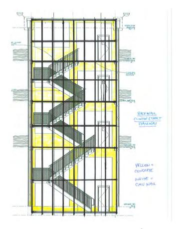
Above: The back wall is comprised of a mix of concrete and CMU (concrete masonry unit). The interior is approx 50' tall x 24' wide. The doors at each level are 3' x 7'. The stairs and handrails will not be attached to the back wall, but will be within 1-2 inches.
