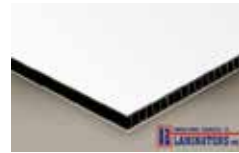
6mm Alupalite - 2-sided sign panel with high gloss baked enamel finish aluminum sheets laminated over a corrugated polyallomer (CPA) core
